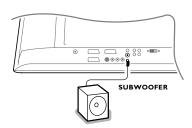
To enhance the sound reproduction of your TV you can connect an externally powered subwoofer (between 20 and 250 Hz).
